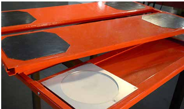
Concave sliding surfaces control seismic response.
