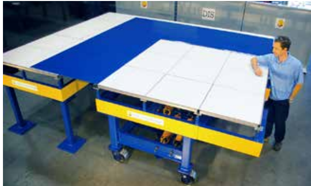
Full scale isolated floor with seismic moat.
