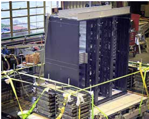
3D shake table testing of DIS' floor isolation system at the University of California, Berkeley.
