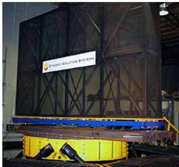
3D shake table testing of DIS' 3D isolation system at Dynamic Certification Laboratories.
