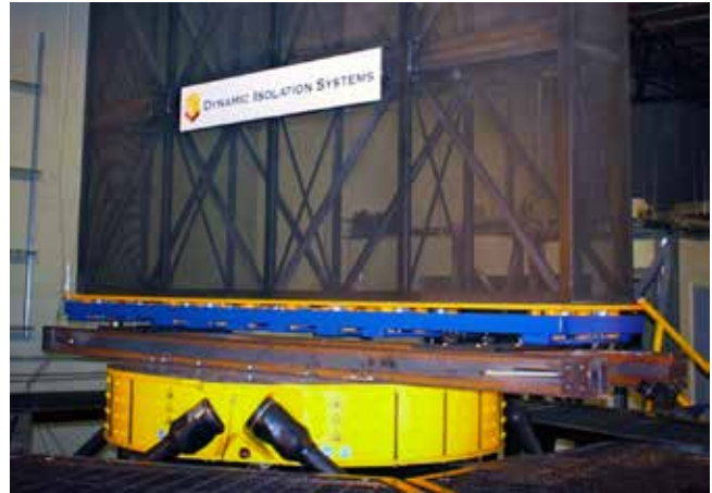
3D shake table testing of DIS' 3D isolation system at DCL.
